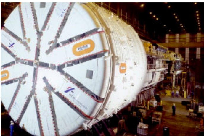
Figure 2: Tunnel boring machine Groene Hart, slurry shield method
