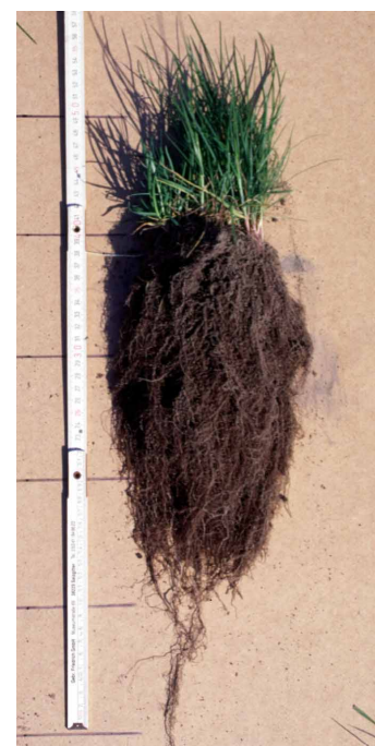
Fig. 2: Root lengths measured one year after grassing of a sandy waste dump (right)
