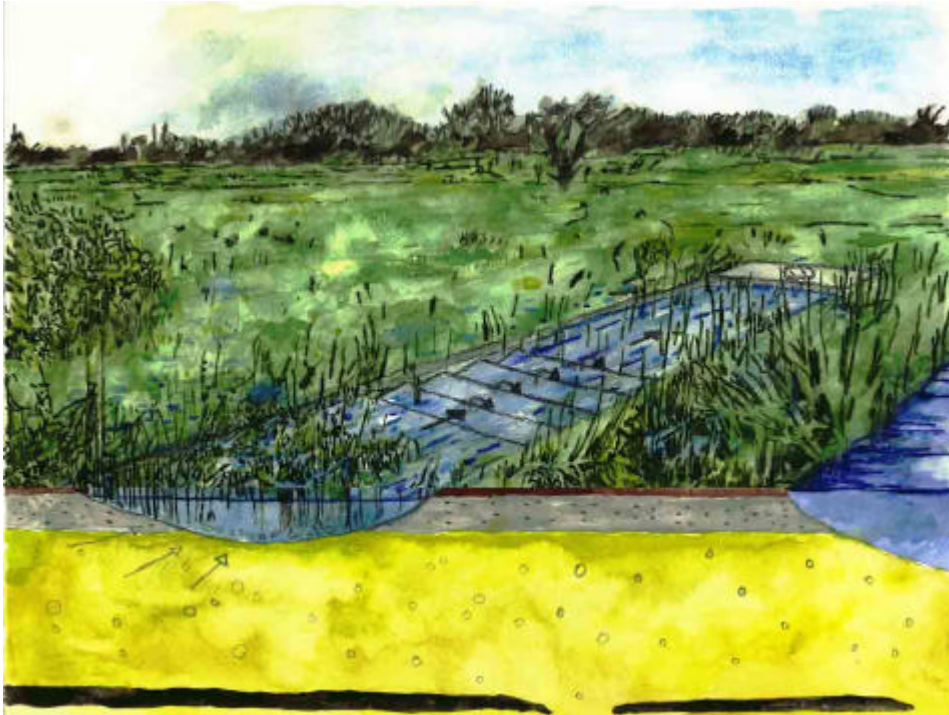
Figure 4. Example of a helophytic filter and cascade system for the aerobic treatment zone.
