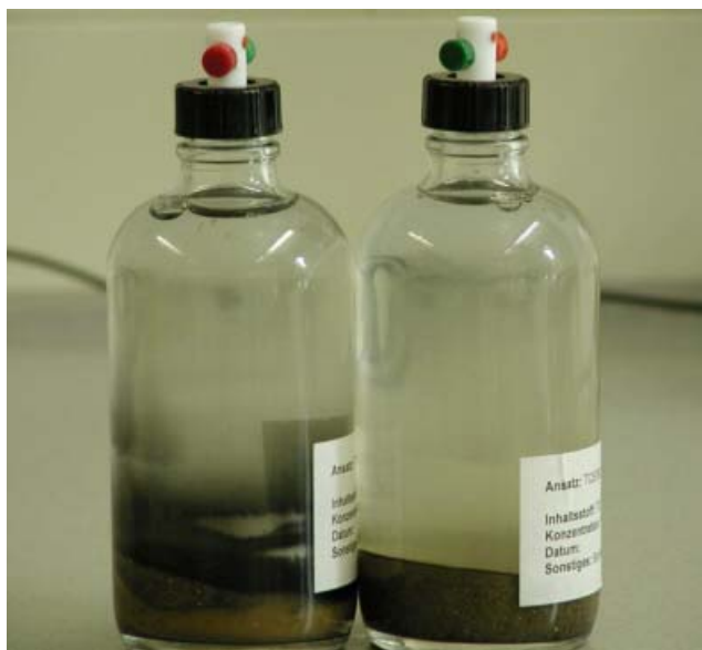
Figure 3: Precipitates of iron sulfide in the "enhanced microcosms" with HRC ® .
