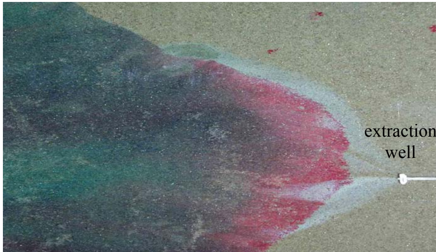
Figure 3: Solubilization and mobilization of a PCE pool (red) with microemulsion (blue-green)
