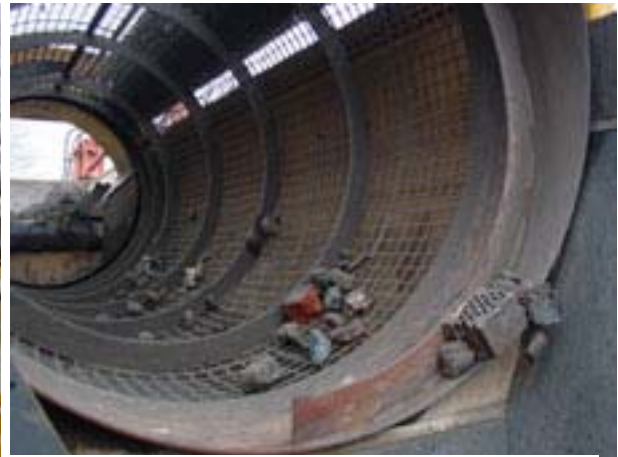
Fig. 7: Sieving of the excavated material
