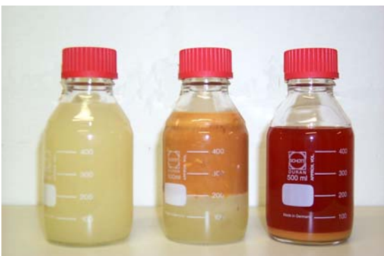
Fig. 3: Microemulsion, diluted (left bottle), and concentrated (right bottle) after evaporation
