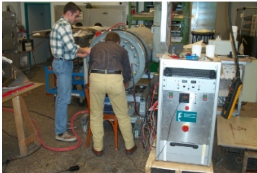
Fig.1: Upgrading a standard autoclave system at DLR Braunschweig with the HEPHAISTOS-Technology
