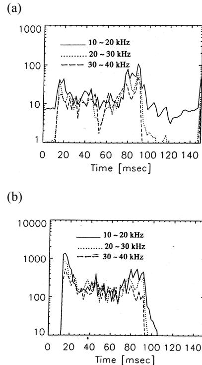
Fig.3 Time evolution of (a) scattered wave power and (b) signal of reflectometry at the frequency of 39 GHz.
