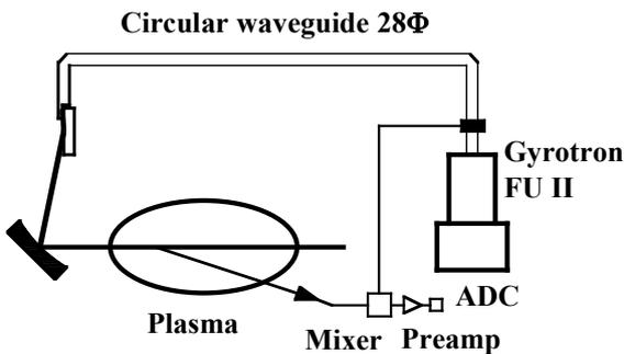
Fig.2 Block diagram of the submillimeter wave scattering measurement.
