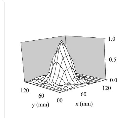
Fig.8 Measured intensity profiles of output beam.
