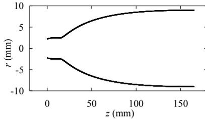
Fig.5 Configuration of the cavity and up-taper.
