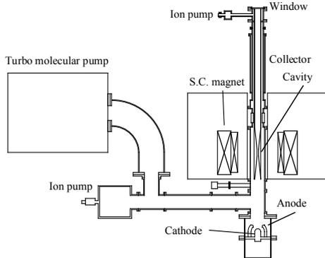
Fig.4 Schematic drawing of Gyrotron FU VA.
