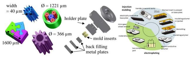
Figure 1: a) examples for polymeric microparts, b) tooling concept for LIGA-mold inserts for the Micro System 50 micro injection molding machine c) Process sequence of the MSG process
