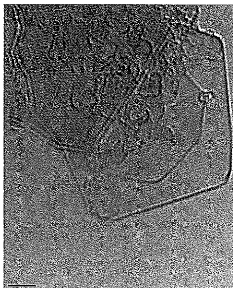
Figure 1. Detail HRTEM view of a graphene and FLG flake.
